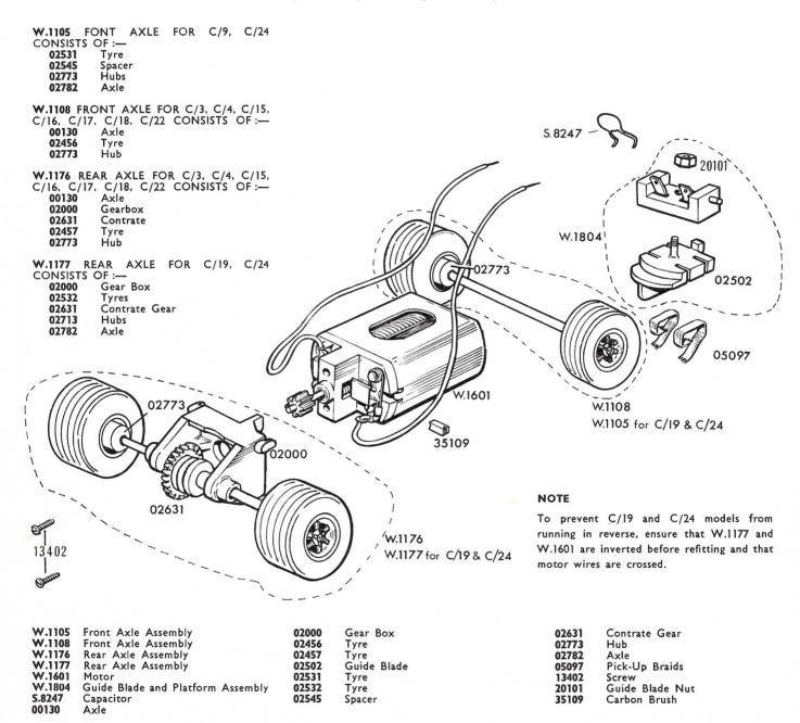
Modifications are made from time to time to Rovex Triang models, If a spare part is required which does not coincide with the illustration, a full description should be given and, if necessary a sketch or sample should accompany the order. The parts which comprise an "X" or "W" assembly are not available as separate items unless the individual parts are numbered.
